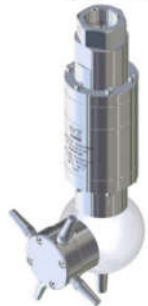
A300 R Option Flows to 300 l/min to 1000 Psi 360° or 240° options
