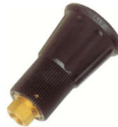
Nozzle Holder with adjustable pressure To 4000Psi - 21 l/min - 60°C Inlet / Outlet - 1/4" BSP F
