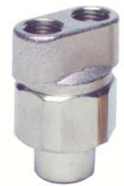
Double Nozzle Holder To 3000Psi - 21 l/min - 60°C Inlet / Outlet (2) - 1/4" BSP F
